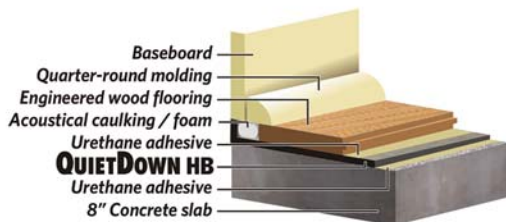
Concrete slab with engineered wood
