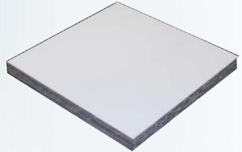
Fabreeka-PTFE bearing pads are used for conditions where it is necessary to accommodate lateral movement (expansion). The PTFE provides a low friction sliding surface on the Fabreeka bearing pad, which distributes high compressive loads and accommodates rotations. In a structural bearing design, polished stainless steel is typically used as the smooth surface that the PTFE slides against.
